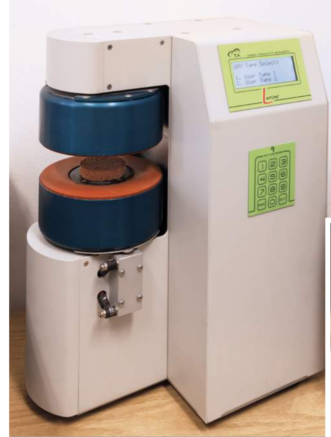
A stationary heat flow meter to study the efficiency of the heat transfer coefficient of materials made of clay and used coffee within the range between 0,1 W/(m·K) and 10 W/(m·K)
