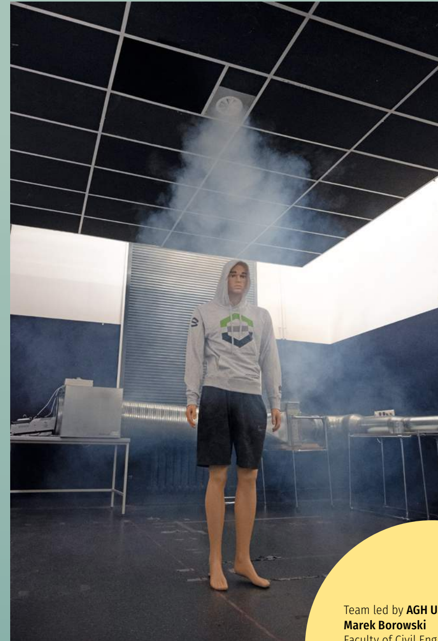
Smoke test used to visualise the propagation of air around the dummy
