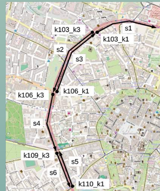
The scope of the dynamic lighting control system (the map shows the northwest bypass of the Krakow city centre) and a fragment of the control graph that manages the data from sensors with dimming parameters of lamps
