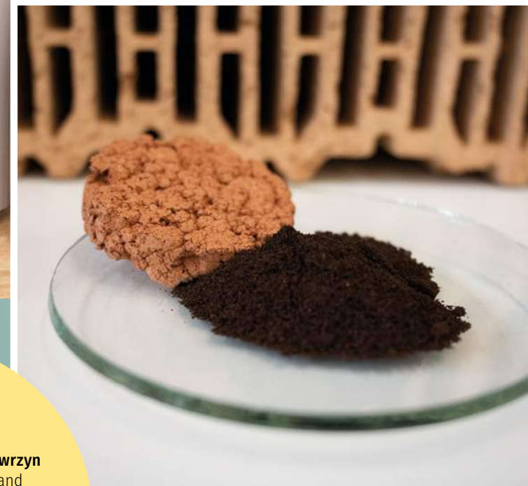
Used coffee grounds and a ceramic material made thereof
