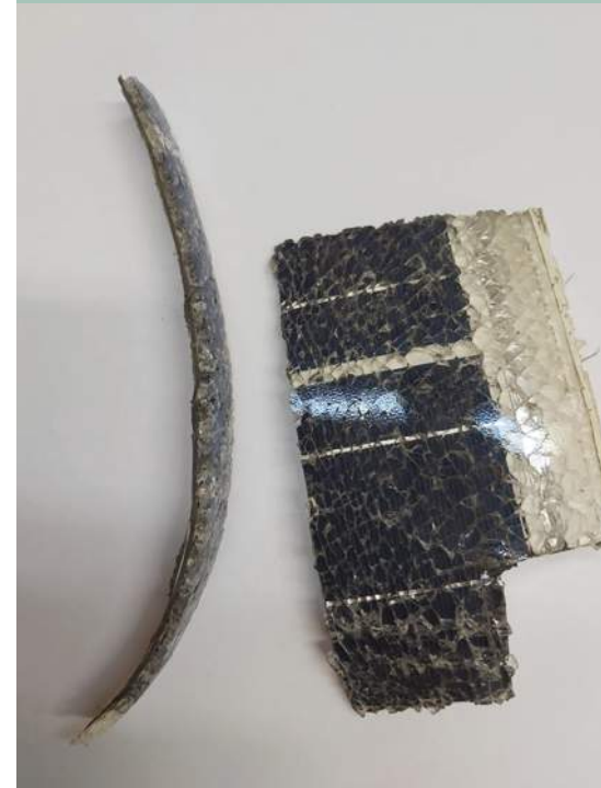
A photovoltaic panel prepared for recycling (with crushed glass layer)
